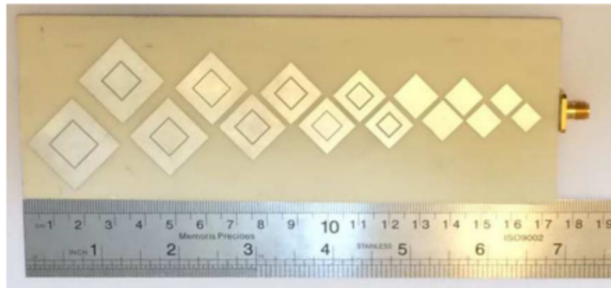
Figure A24: Fabricated Log-Periodic Fractal Antenna Configuration (Courtesy Amini, A., et al.)
