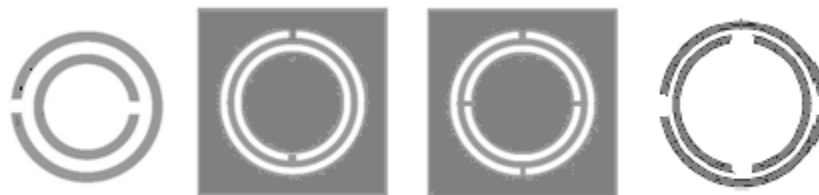
Figure App 1: Split Ring Resonators (SRR, CSRR, DS-CSRR, DS-SRR) (Courtesy Jindal, S. and Sharma, J.)
