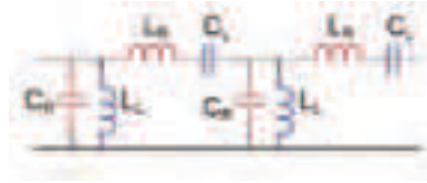
Figure App 6. Equivalent Circuit Model of Composite Right/Left-Handed Transmission Line (Courtesy Jindal, S. and Sharma, J.)
